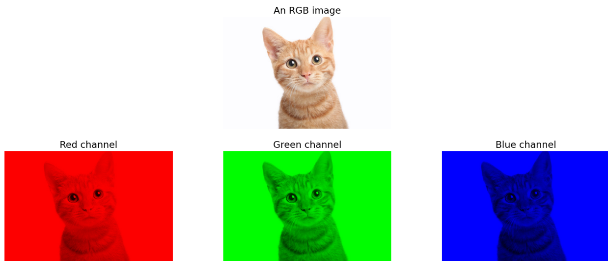
Fig. 6.1: An image and its 3 channels (Red, Green and Blue intensity, from left to right).
